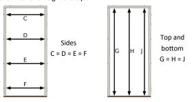
Also check that the frame is plumb inwards and out, and that it is not twisted in any way.
