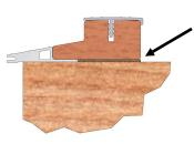
Use the lowest two straps to fixate the threshold, centred and level.
