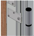
Re-torque the screws in the frame hinges and make sure their locking screws are tightened. Instructional videos on this is available on our website.
