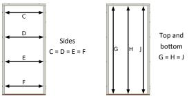
Also check that the frame is plumb inwards and out, and that it is not twisted in any way.
